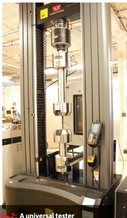
FIG. 2: A universal tester measures tensile and other properties of composite materials for specified geometries.
