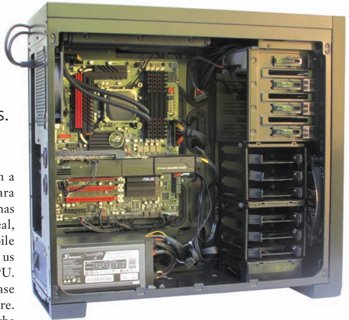
The interior of the Kronos 800S. Note the liquid cooling system, as well as the two USB cables routed to rear USB ports to activate the USB 3.0 ports in the front panel. Image courtesy of David Cohn.
