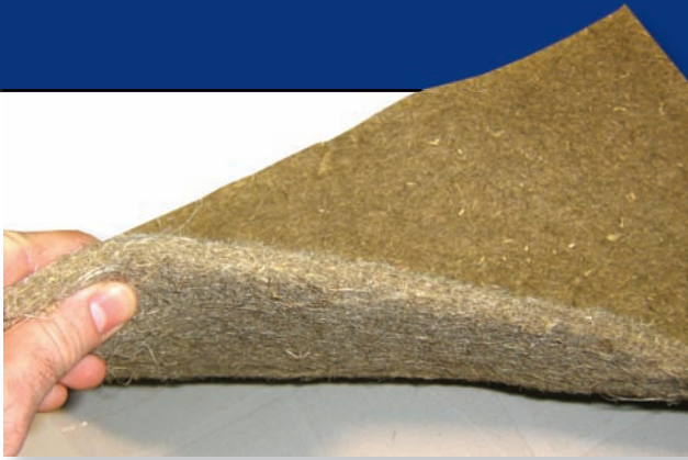
Non-woven biofiber mat is used as composite reinforcement.
