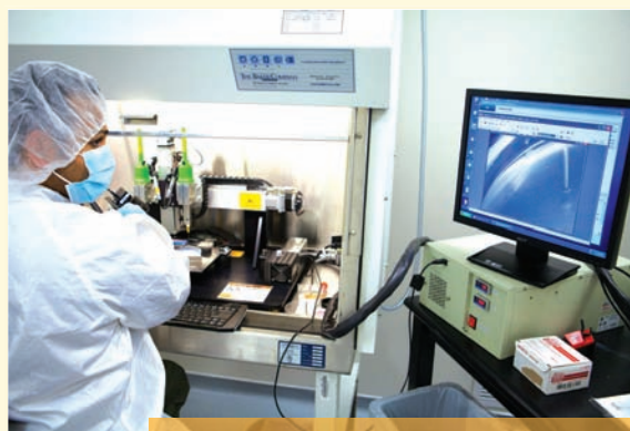
One of Organovo's tissue engineers oversees the construction of a vascular tissue construct on the Novogen MMX Bioprinter. Image courtesy of Organovo.
