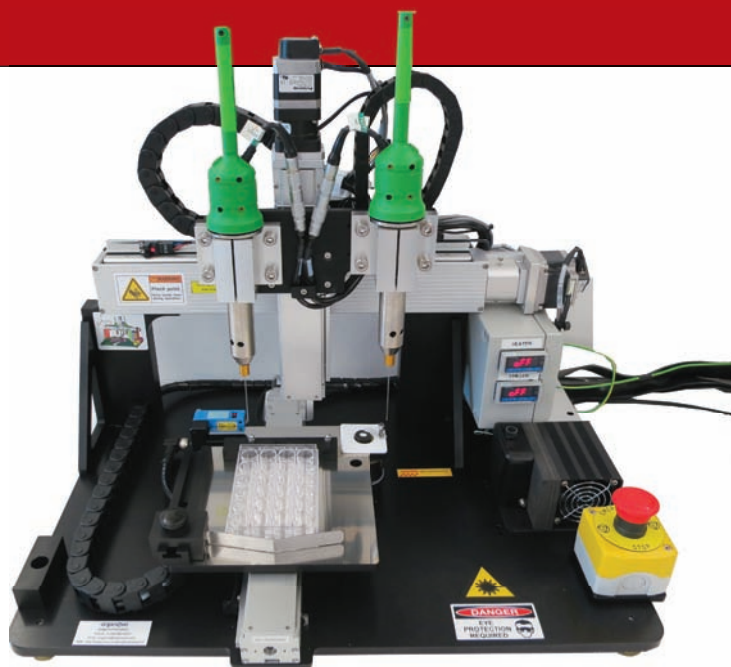
The Novogen MMX Bioprinter prints fully human, architecturally correct 3D tissue in a variety of different formats — in this particular case, into multi-well plates. Bio-ink or hydrogel can be dispensed from each of two printheads. Image courtesy of Organovo.
