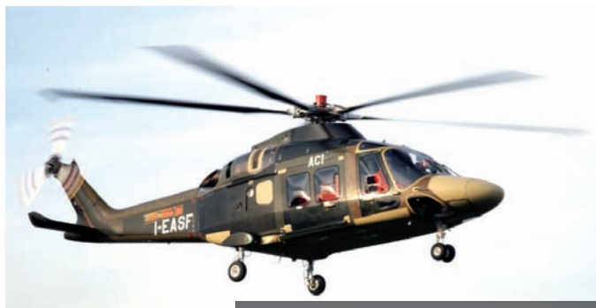
FIG. 1: As a new generation of helicopter technology, the AgustaWestland AW169 horizontal tailplane has a length of 9 ft. and uses thermoplastic material, a high-performance engineering polymer and carbon/polyphenylene sulfide (PPS) semipreg and plate material. Image courtesy of AgustaWestland.
