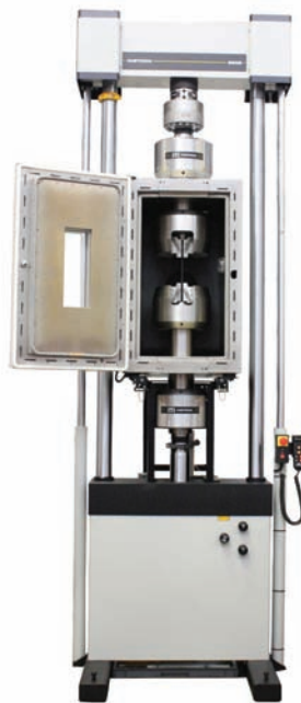
FIG. 4: Instron hydraulic and electrodynamic fatigue testing machines allow customers to conduct fatigue tests. Image courtesy of Instron.
